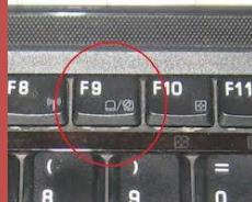
**Functions Keys** are the keys used to execute different and specific functions. They are tagged F1, F2, F3, etc. Up to F12. The function of each key is different according to the program.
