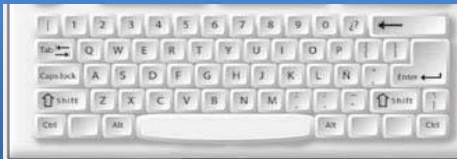
**The alphanumeric keyboard** is similar to the typewriter. It has the keys for the alphabet, the numbers from 0 to 9 and the punctuation and stress signs
